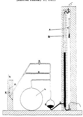
A Variable Resistance.—The following is a description of a variable resistance which has several advantages over the ordinary slide wire resistance. The accompanying diagram illustrates the instrument.
